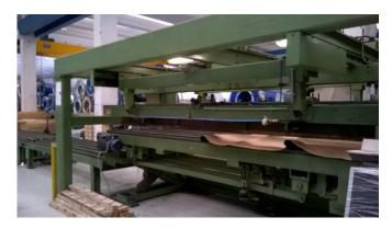
Three unloading catenaries that can be controlled from both the main pulpit and the strapping station (4000 mm each); second equipped with chains and third with weighing machine
